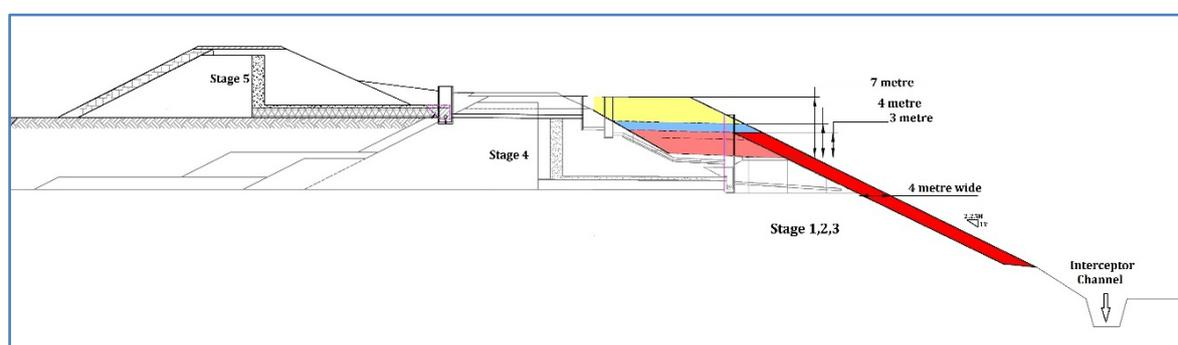
**Figure 9.1** Cross section of facility embankment with proposed buttress
